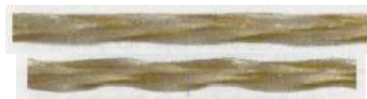
Fig. 2. Auxetic yarns, polyamide/cotton
