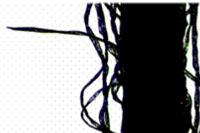
b) flattened yarn with loading 25 N
