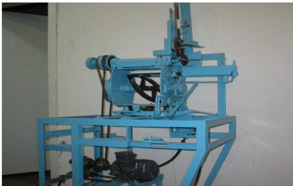
Picture.3. Kinematic scheme of winding head for the formation of TTF of undersize dimensions with the wedge gear for movements of thread guide pusher
