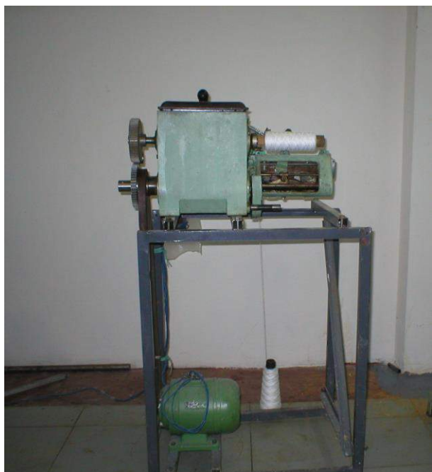
Picture 5. External appearance of winding head for formation of TTF of undersize dimensions with the reduced stroke of the thread guide
