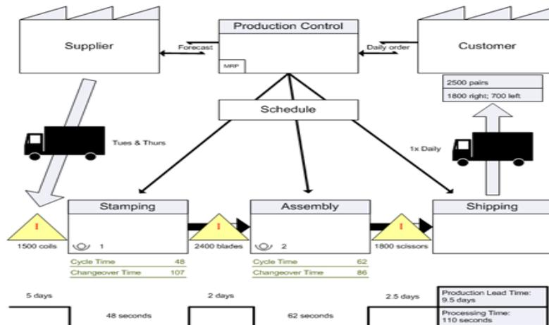
Picture 3. Measurement and design of the process by means of the Value Stream Mapping Method – simplified diagram.
